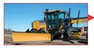
Blade has a 12' cutting edge, 30" intake and a 40" discharge.
