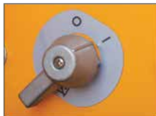
BATTERY DISCONNECT SWITCH
